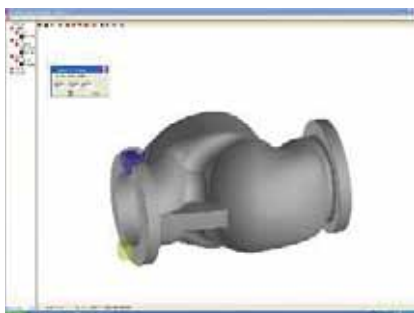
Riser and chill added to the casting model using component parts.
