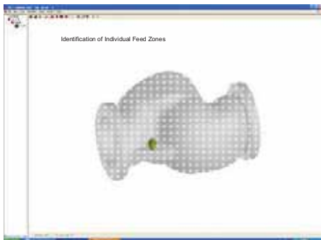
Feeding paths on the valve body casting, along with last points to freeze in various feeding zones.
