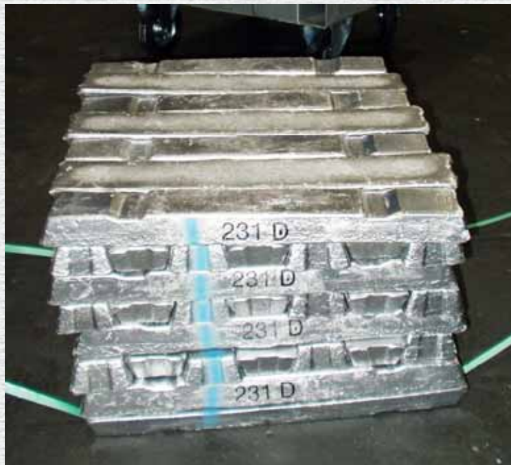
block material: 6 kg ingots
