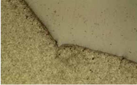
Figure 4: Gathering of the porosities close to the interface (100x magnification no etching)
