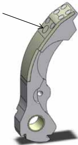
Figure 1: Dedicated rifle component. Arrow shows the impact direction. Blue region is base metal (ZAMAK 7) and gray region represents steel insert
