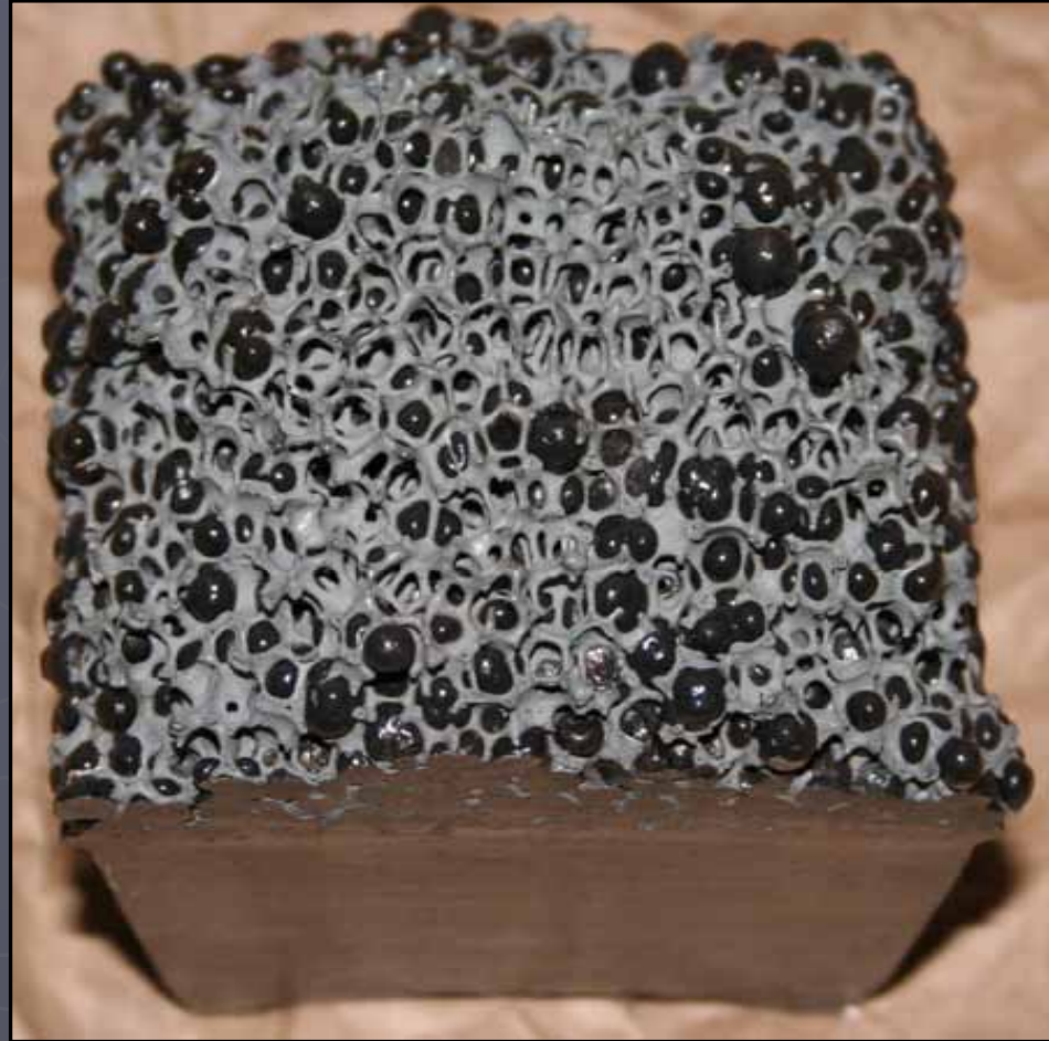
Fig. 3a : "Blocked Filter". View from below.
