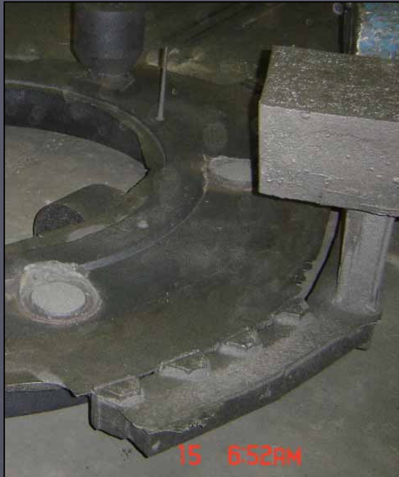
Figure 12 : Impurities in front of the filters and on top of the pouring basin.
