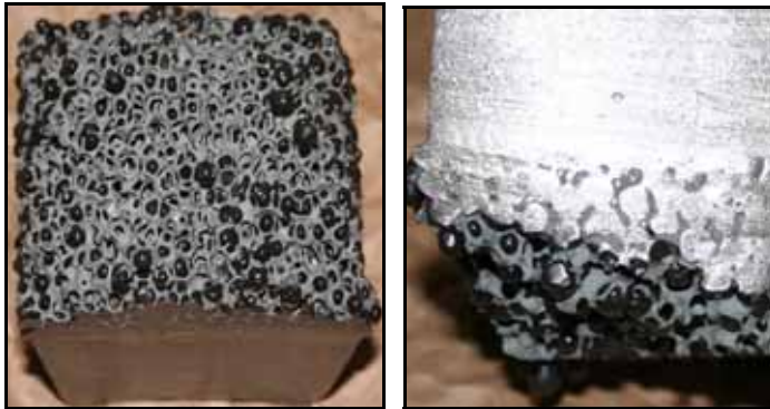
Figure 3 : “Blocked Filter”. View from below and side view.
